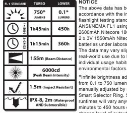
The above data has been measured in accordance with the international flashlight testing standards ANSI/NEMA FL1 using one x 3.7V 2600mAh Nitecore 18650 battery and 2 x 3V 1550mAh Nitecore CR123 batteries under laboratory conditions. The data may vary slightly during real-world use due to battery type, individual usage habits and
